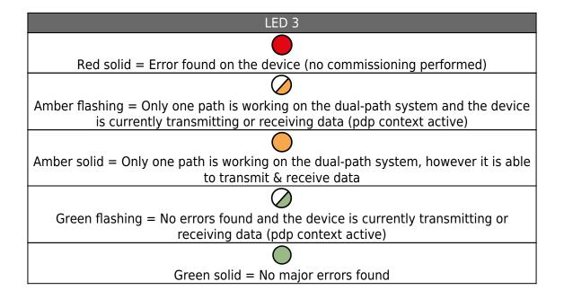
Figure 11 - Connectivity Section
