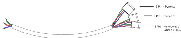
Figure 9 - Serial Cable (RS232/485/TTL)
