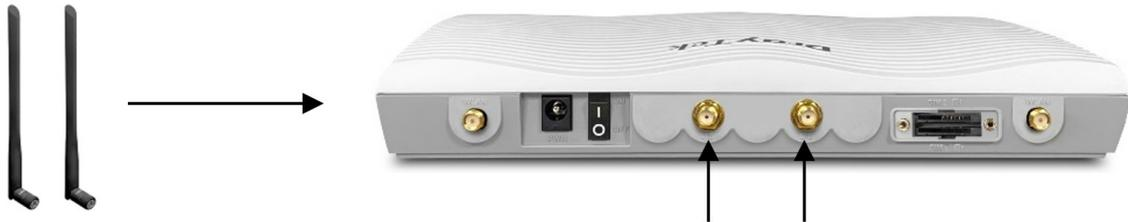
3. Whilst optional, the antenna-to-extension base installation is recommended for improved mobile signal strength. Screw the antennas into the extension bases.
